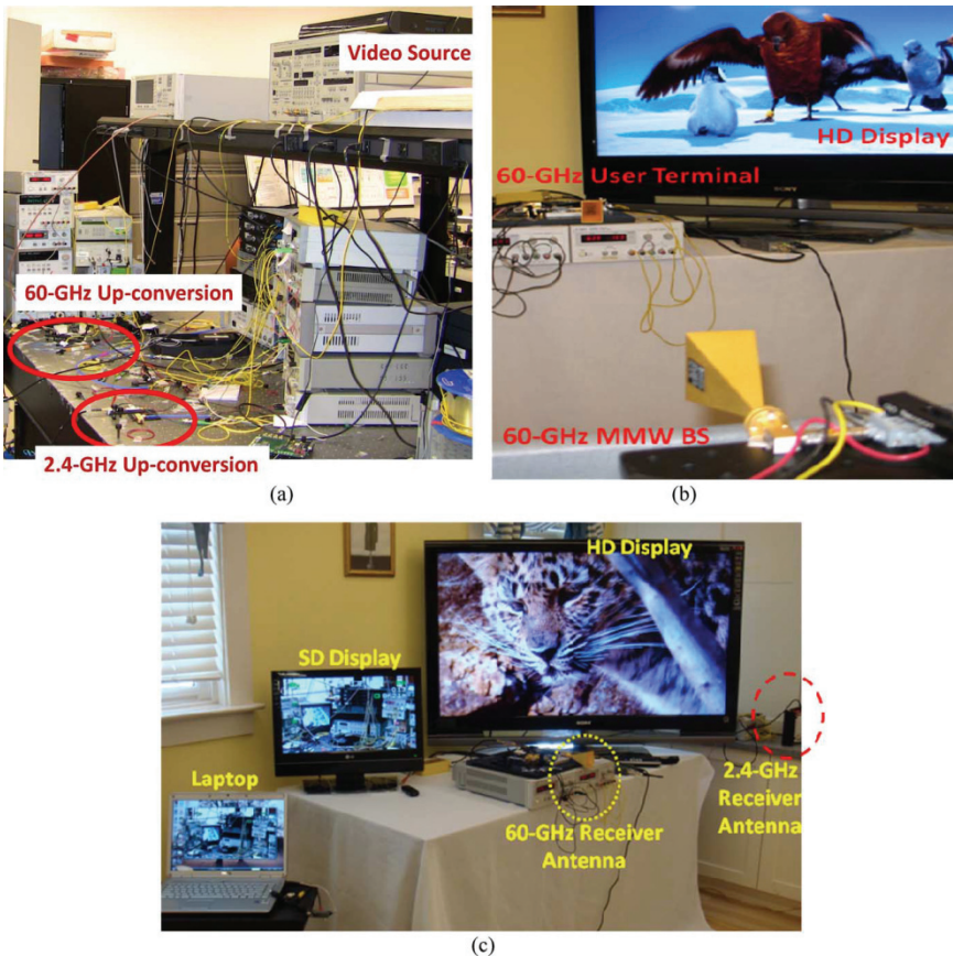
Fig. 39. Transmitter and receiver of the 3-screen, dual-service 2.4-GHz and 60-GHz RoF carrying 270-Mbps SD and 1.485-Gbps HD video content. (a) Transmitter at Centergy lab at 10th Street, (b) 60-GHz Wireless setup at residential lab at 5th Street, and (c) 3-screen receiver at residential lab.
